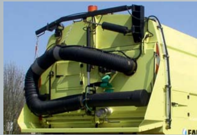
Manual suction system at the rear
